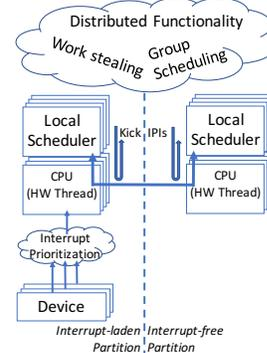
**Figure 1: The global scheduler is a very loosely coupled collection of local schedulers, one per hardware thread/CPU. Most CPUs are “interrupt-free” and see only scheduling-related interrupts. All CPUs are subject to SMIs at all times.**
