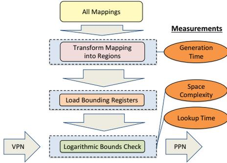
Fig. 14. Address translation by registered multiplexor tree.
