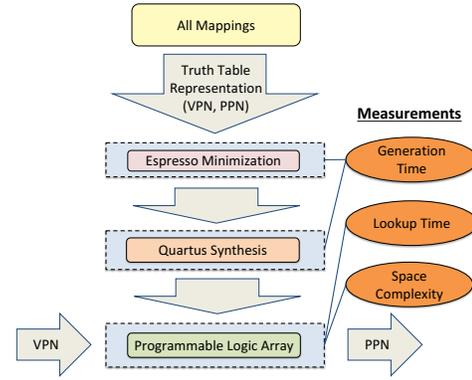
Fig. 8. Functional address translation via Espresso-minimized PLAs.
