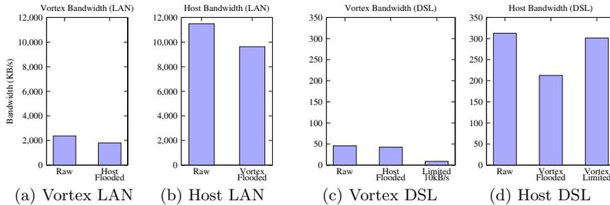
**Fig. 8.** Bandwidth measurements of clients hosted on DSL and LAN connections. (a) and (c) contain the performance results of a Vortex CSW, while (b) and (d) contain the performance results of the client machine. Measurements were taken under various traffic conditions and bandwidth is measured in kilobytes/second. Each figure shows the mean taken from 10 separate trials.
