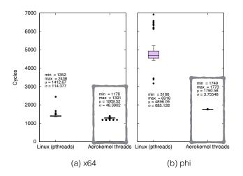
Figure 3: Thread context switch latency. Aerokernel thread context switches similar in average performance to Linux on x64 and over two times faster on Phi. In both cases, the variance is considerably lower.
