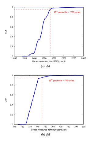
Figure 5: CDF of IPI one-way latencies, the hardware limit of asynchronous signaling that is available to HRTs.
