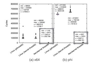
Figure 2: Thread creation latency. Aerokernel thread creations are on average two orders of magnitude faster that Linux userspace (pthreads) or kernel thread creations and have at least an order of magnitude lower variance.
