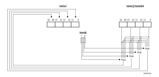
Table 1-20. Immediate-Byte Operand Encoding for PSHUFW
