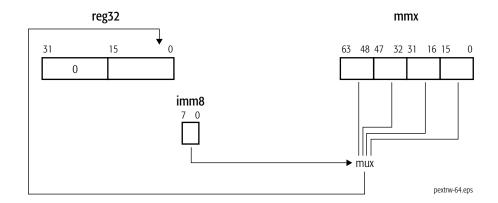
Table 1-1. Immediate-Byte Operand Encoding for 64-Bit PEXTRW
