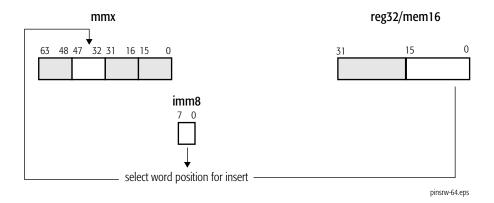
Table 1-19. Immediate-Byte Operand Encoding for 64-Bit PINSRW
